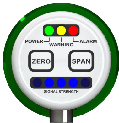
Figure 6-7: Automatic Span calibration accepted
