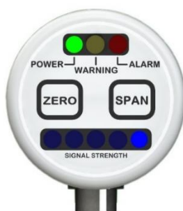
Figure 6-2: Illustration of the strongest signal → no obstructions to the light beam
