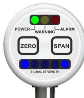
Figure 6-11: Auto span calibration ready to start after the zero calibration is complete
