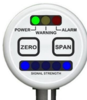
Figure 6-14: Signal Strength LEDs showing when to release ZERO to enter Service Mode
