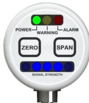
Figure 6-12: Signal Strength LEDs indicate successful Auto SPAN Calibration
