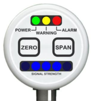
Figure 5-2: Laser beam has been blocked – Auto Span calibration registering
