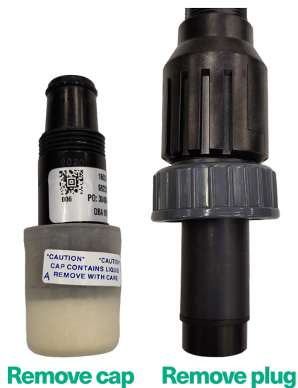
Figure 6.2: pH electrode installation
