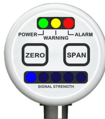
Figure 7-3: Illustration of the weakest signal → obstructions to the light beam
