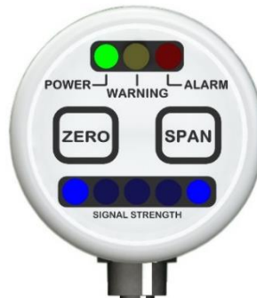
Figure 7-6: Auto span calibration ready to start after the zero calibration is complete (left and right SIGNAL STRENGTH LEDs illuminated)
