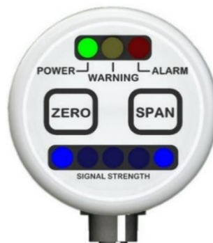
Figure 7-9: Signal Strength LEDs showing when to release ZERO to enter Service Mode
