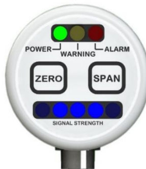
Figure 7-7: Signal Strength LEDs indicate successful Auto SPAN Calibration
